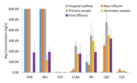
Figure 1: Average (avg) concentrations of pharmaceuticals in ng/L detected at separate stages of the wastewater treatment process. Error bars indicate standard deviation (n=7). PAR = paracetamol, IBU = ibuprofen, DCF = diclofenac, CLAR = clarithromycin, TRI = trimethoprim, CBZ = carbamazepine, FLX = fluoxetine.
