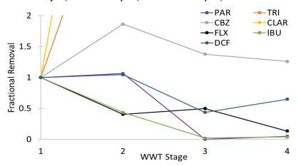
Figure 2: Fractional removal of pharmaceuticals at separate stages of the wastewater treatment process. 1 = raw influent, 2 = primary stage, 3 = secondary stage, 4 = final effluent.
